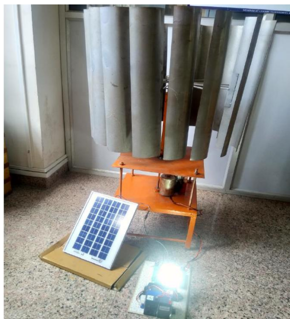
Fig8: Whole set-up of VAWT and solar panel
